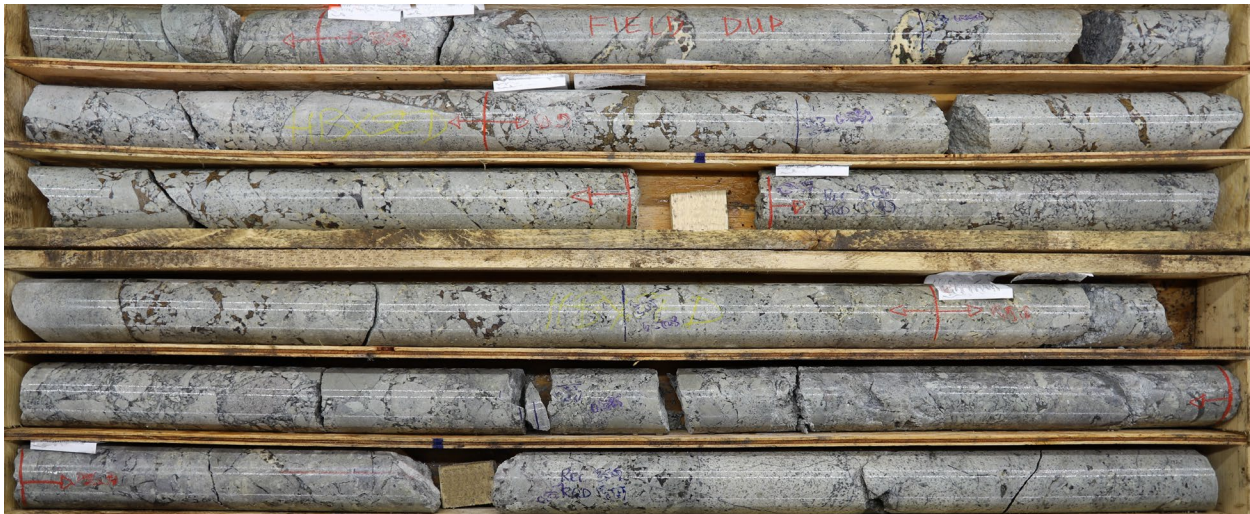
Figure 2. Example of near-surface, sphalerite-cemented hydrothermal breccia from BK21-060 at 50.5 metres downhole.
