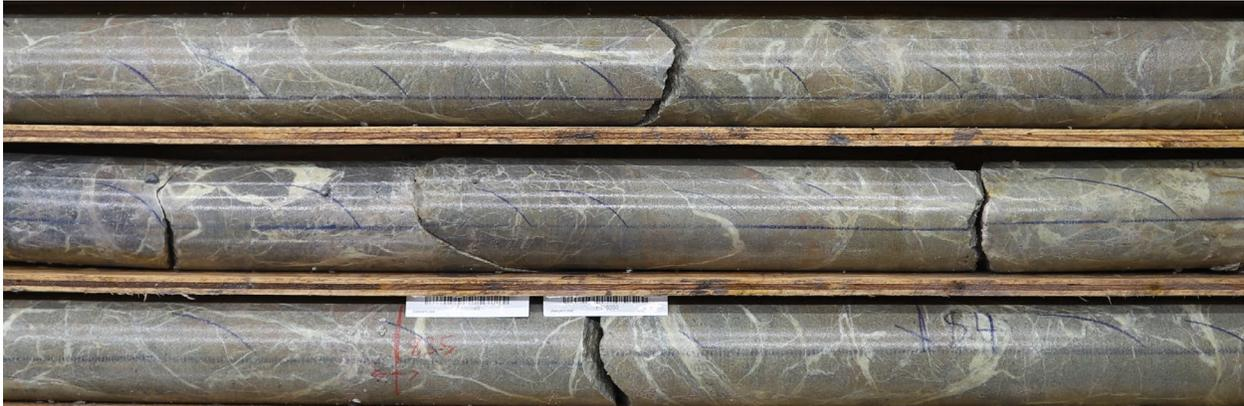
*[Figure 1: Strong hydrothermal-related alteration with quartz-pyrite veins in IRK23-001](#)*
