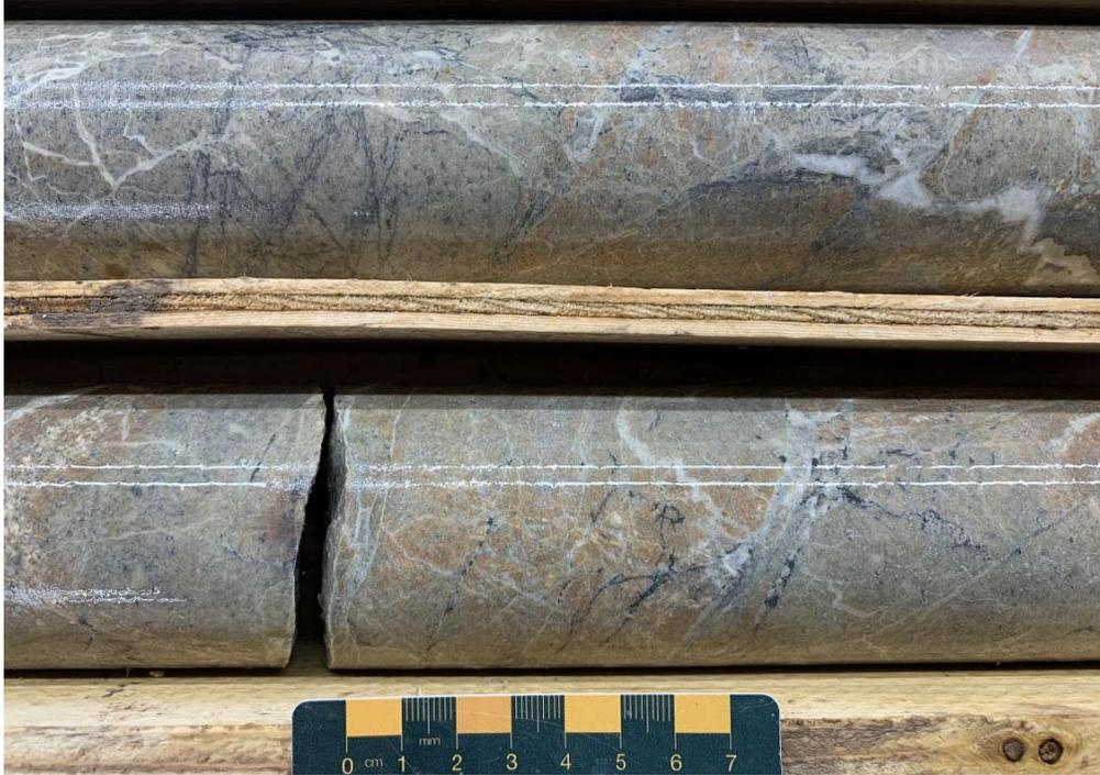
[Figure 2: Veining in a fine grained equigranular intrusive rock with fine black sulfides in quartz-carbonate veining in IRK23-005. pXRF analysis of these sulphides indicate elevated Ag, Cu, Pb, and Zn.](#)
